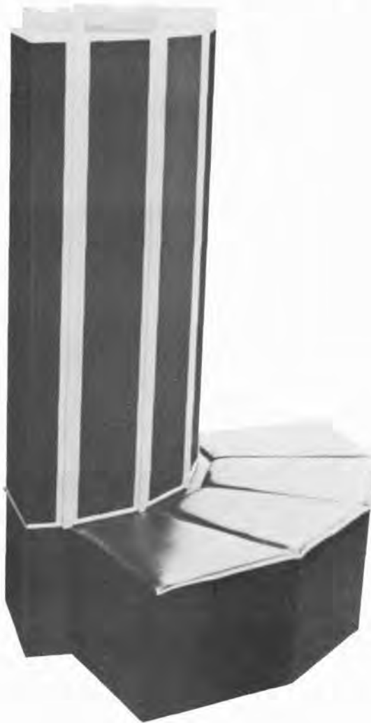
Figure 1-5. I/O Subsystem chassis
