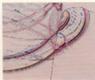
Left, wavefield snapshots inside salt diapher. Images show how energy is reflected or refracted by subsurface geology.
