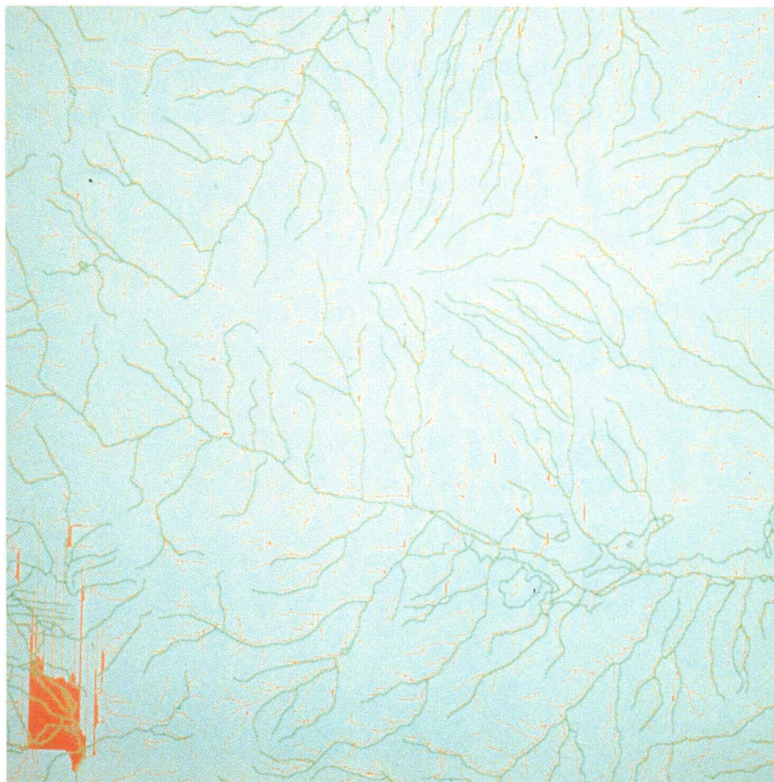
Figure 3. Anomalies, such as that in the lower left corner, must be identified as either a defect in the DEM data, an artifact of processing, or a valid feature. After identification and possible correction, processing is restarted.
