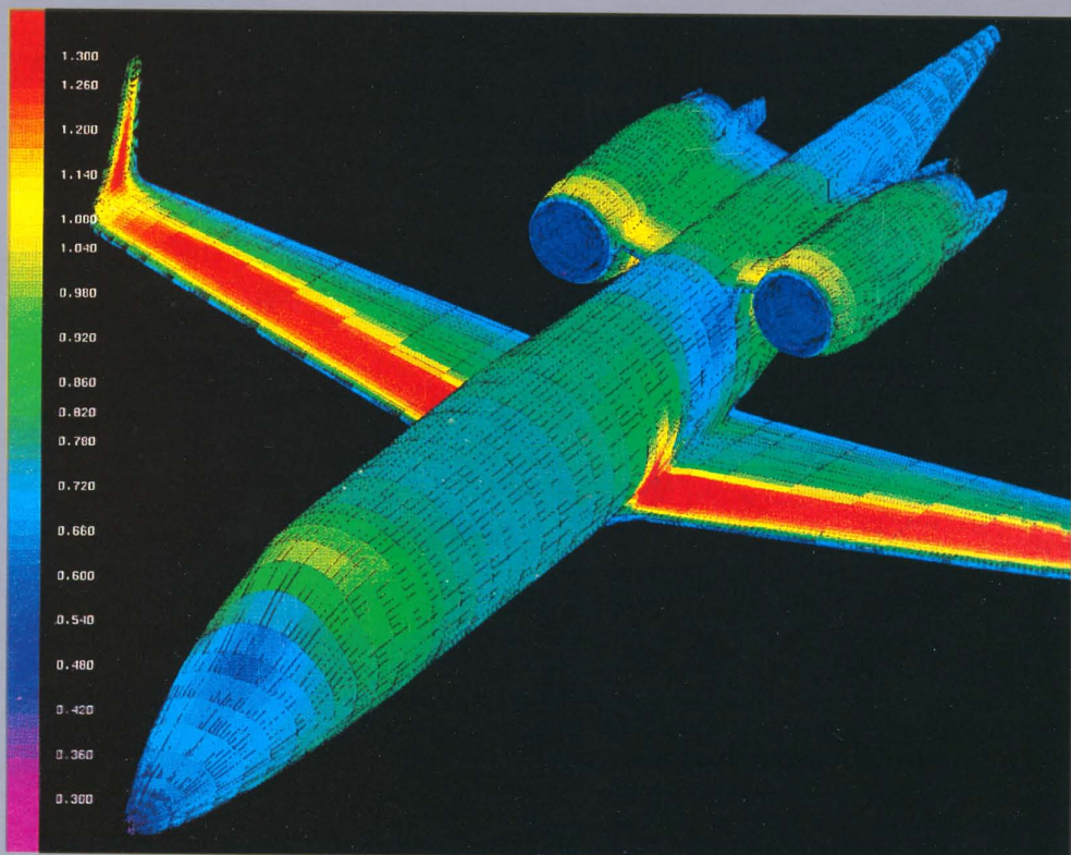
(Below). Aerodynamic shock waves across the wings and fuselage as modeled on Learjet Model 60. Yellow represents barely supersonic and red is Mach 1.3.
